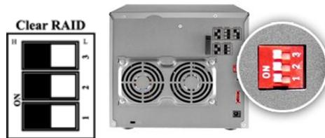
3. Simultaneously press "**reset button**" and "**power button**" until there is a beep sound. When DIGIARRAY powers on with a beep sound, the RAID configuration is done.
